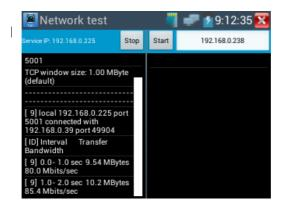
2. Start send packet test::Using the other IP tester and type in the Server's IP address at the top right corner of the screen. This app is used to send packets for network speed testing. Click the "Start" button to send the packets and start testing.
