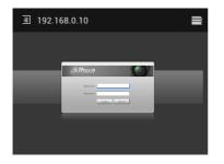
The IP camera and IP tester must be on the same network segment for the browser to interface with the camera. If they are not in the same segment, click the button or press "RETRUN" to exit. Open the "Settings" app from the main menu to change the IP tester's network settings to match those of the IP camera.
