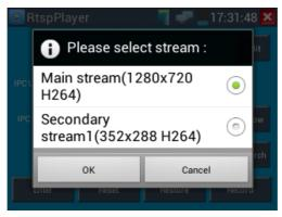
Note: in the event the ip tester does not auto detect the rtsp stream, refer to the specific camera manufacturer for the specific rtsp stream url. you may find this on line with a search of the camera model number and the word rtsp.
