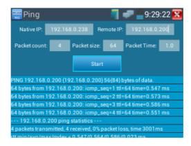
**Application:** PING testing is the most conventional network debugging tools. It is used for testing if the connected IP camera or other network equipment's Ethernet port is working normally and the IP address is correct.
