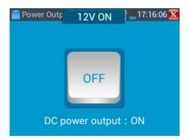
1 .Don't input any power into the "DC12/1A OUTPUT" port of the IP camera tester to avoid destroy.
