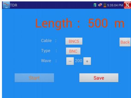
3. Click “+” or “-” to adjust wave speed, while display length is the same as the actual Length, click “save” to save calibration data, It can be used for the same cable testing after the calibration.
