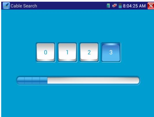
Turn on the cable scan; use the copper pin to search, the cable with loudest voice means it is connected with the tester. Four Audio types can choose. LED lamp is convenient to work in dark or at night. Press the button (+ -) to adjust the volume, use two batteries (size AAA)
