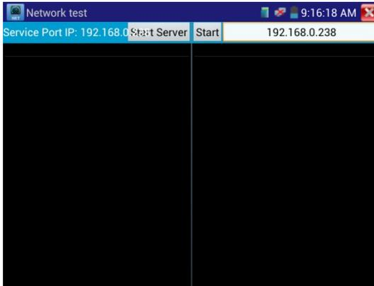
When test , need a Instrument or Network Test Software as the Server, another one send packet test . The two instruments must be in the same network.
