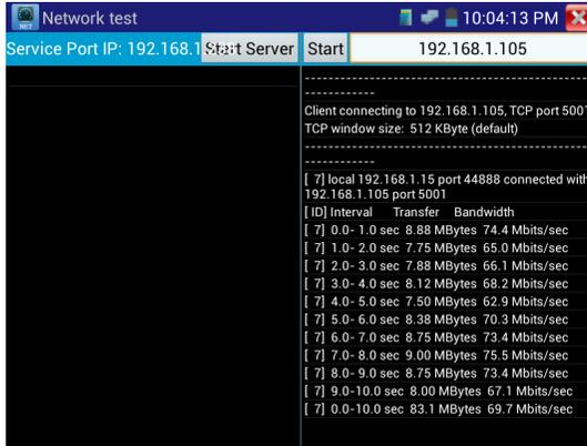
Or Instrument as the server, computer as test client ( select client, fill instrument IP address to test )
