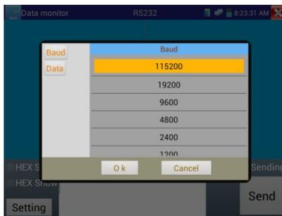
Click “Set” to choose the baud rate of RS485/RS232; it must be the same as the DVR or the Control keyboard . The DVR or Control keyboard send the code to the tester, if it can be read, the protocol will shown on the upper right, like Pelco D, if not, like P:---
