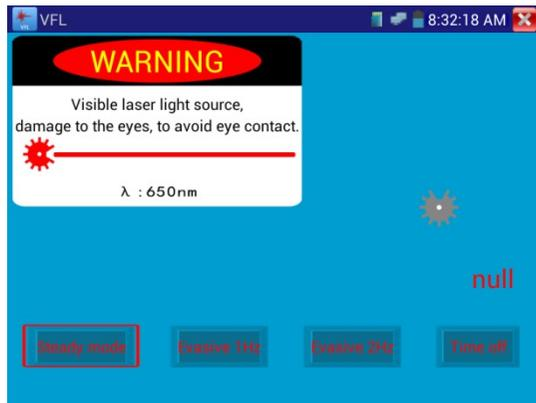
VFL four status can select——“Steady mode”, “Evasive 1Hz”, “Evasive 2Hz”and“Time off”. Click button “Steady mode” to enter steady status, click button “Evasive 1Hz” and “Evasive 2Hz, to enter pulse mode, click button “Time off”, VFL be turned off. Timed turn off can select (5mins, 10mins,
