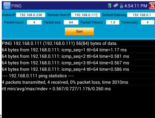
**Application:** PING test is used for testing if the connected IP camera or other network equipment’s Ethernet port is working normally and the IP address is correct.
