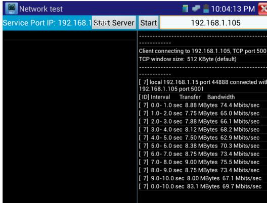
Network bandwidth testing , can be test with an instrument and computer, Install network bandwidth testing software on a computer, As a test client or server , with instrument mutual -testing
