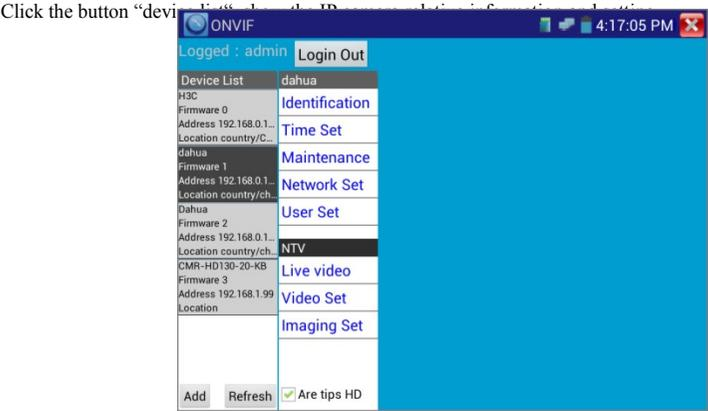
Input IP camera user name and pass word to login, click “Device list” and select the camera to set (device setting, time setting, maintain ,network setting, user management, video live , video streaming, image set etc).Some function operation need IP camera’s authorization.
