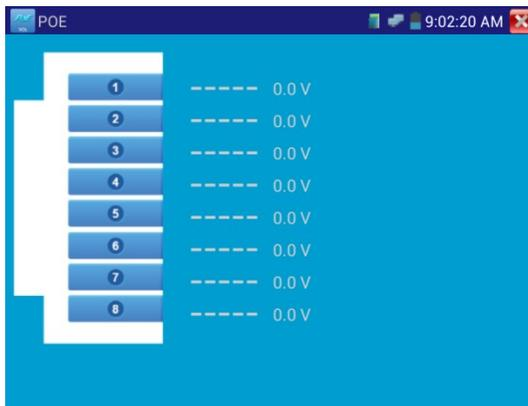
Connect the cable to the power supply equipment's POE port and the tester's PSE IN port. Connect IP camera or wireless AP equipment connect tester's LAN port, the POE voltage and the cable's connection status show on the screen.
