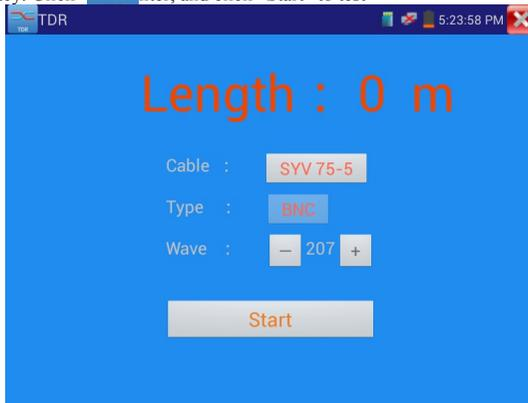
Built-in BNC, network cable, RVV control cable, Telephone line can test. 11 groups user-defined cable can be set.
