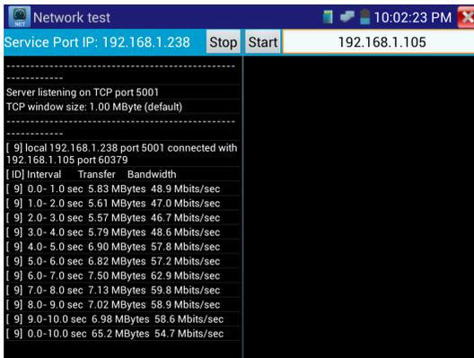
2. Start send packet test: Fill server's IP address in sending packet test, click button “start test”
