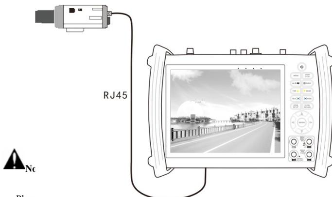
a. Please make sure the connect cable to RJ45 port of PoE power output is straight line, otherwise will damage the tester
