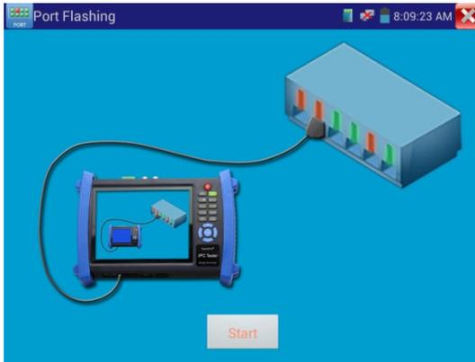
If connect well, the LAN port flash at special frequency, If not, no any changes on the LAN port
