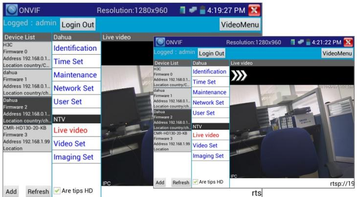
**PTZ control:** click the image to slip left, right, up, down, or zoom in or zoom out, IP dome camera rotate correspondingly, PTZ direction of rotation show on upper left corner.
