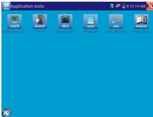
**Audio Record:** Recording and play the received audio. Connect the audio devices to Audio input port, click
