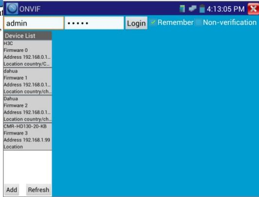
Some IP cameras cannot be Auto scan, select manual scan to add camera, click bottom left “add”, users can add camera manually, URL address should be the ONVIF camera service address.
