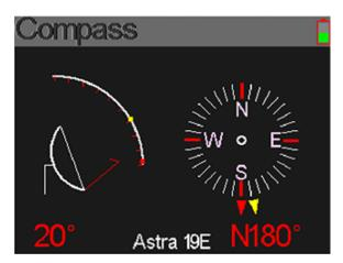
Select Compass and press [OK] to go to compass submenu. And the menu as bellowing figure.
