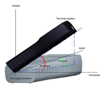
The meter must face to the satellite in the sky that user is plan to find. Belowing is the figure of aligment on this menu.
