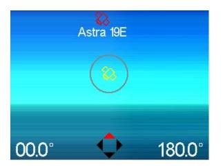
User need to adjust the attitude of the meter according to the simulated results until the current simulated values very close to the right ones. As close as possible. Then the BLUE lines will turn GREEN. Belowing is the graph for meter during adjust.
