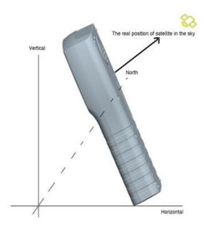
User need to adjust the attitude of the meter according BLUE arraw on the screen. The meter will deep and the RED icon turns to GREEN if the RED icon closes to the YELLOW one. It is better to make the two icon overlapping. And also values of azimuth and elevation will refresh on time according to the current position during the whole process.
