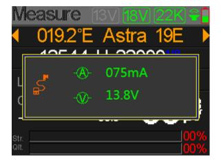
Press F2 to enter into feed current and voltage of LNB measurement menu as below.
