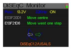
**Pow:** The power supply of the input cable line.
