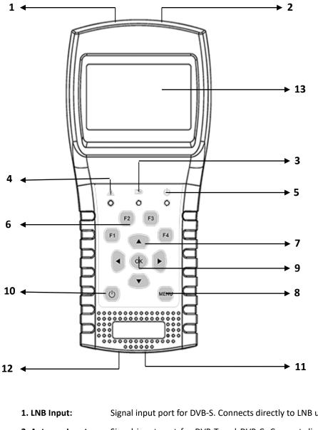
Signal input port for DVB-S. Connects directly to LNB using coaxial cable.
