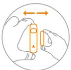
2. Connecting PIR sensor to control panel: power on or trigger the PIR sensor.
