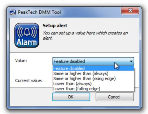
You can define whether the alarm is triggered every time as soon as a measured value exceeds the set range / drops below or only when the measured value increases [rising edge] or decreases [falling edge].
