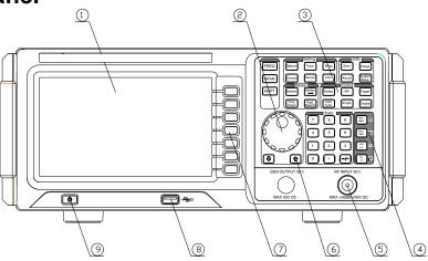
1 LCD display screen 2 Adjusting knob 3 Function key area 4 Digit keys 5 RF input
